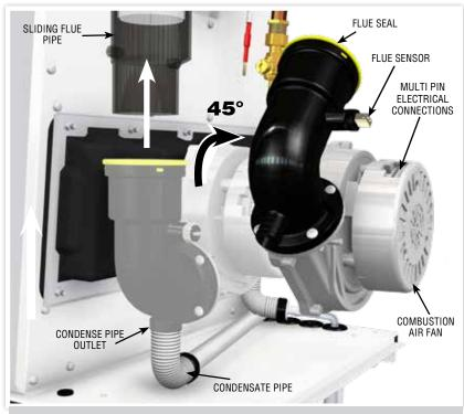
FIGURE 20. COMBUSTION AIR FAN REMOVAL
