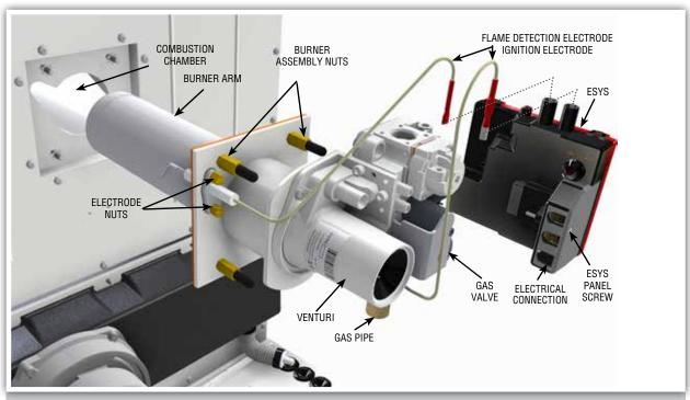
FIGURE 18. MAIN BURNER ASSEMBLY REMOVAL
