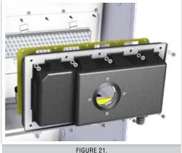
FIGURE 21. COMBUSTION AIR PASSAGE REMOVAL
